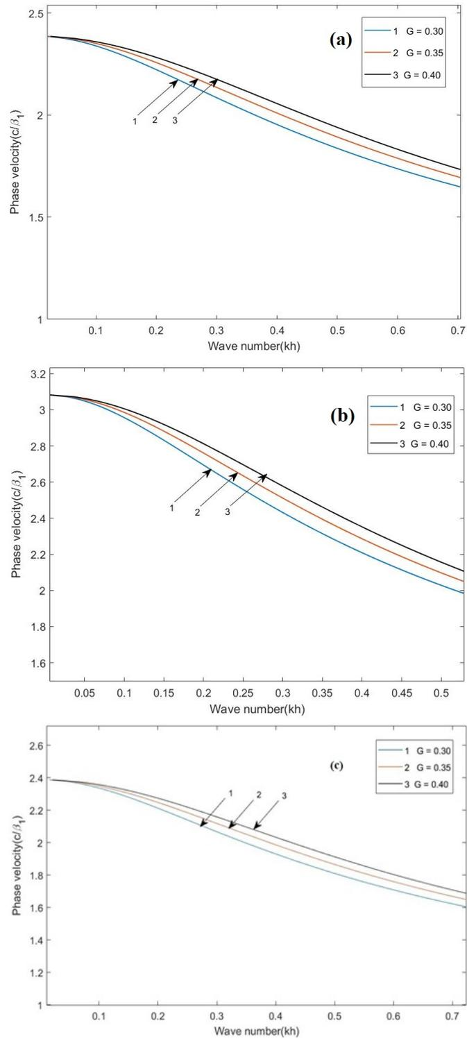
**FIGURE 2.** Imperfectness parameter effects in wave number domain in (a) initial stress presence (b) initial stress absence (c) for  $\eta_1, \eta_2 = 1$ , i.e. when dry sandy layers become isotropic
